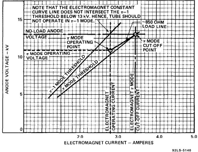
Figure 8 -  $\pi$ -Mode Threshold Characteristics, 850-ohm Load Line
