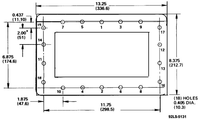
Figure 13 - AJ2192 Flange to Mate CPR975F
