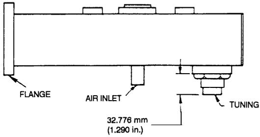
Figure 11 - AJ2192 Waveguide Transition
