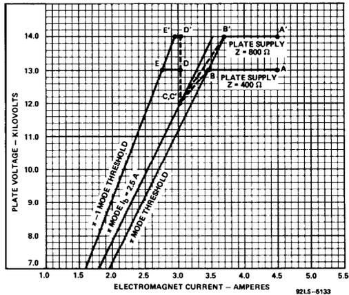
Figure 3 - RF Mode Characteristics
