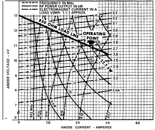
Figure 7 - Performance Characteristics, 850-ohm Load Line
