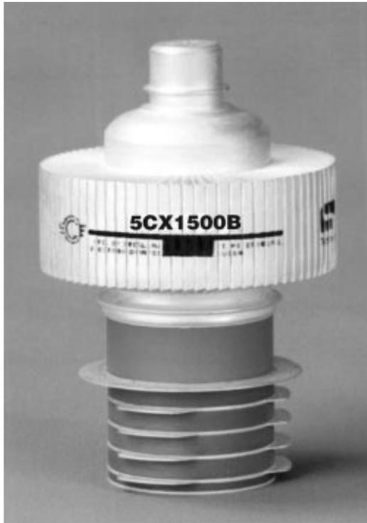
**T**he Svetlana 5CX1500B is a high-performance ceramic/metal power pentode designed for use as a highly linear Class AB<sub>1</sub> linear amplifier. The pentode is ideal for VHF service and is recommended for use in FM broadcast transmitters. The 5CX1500B filament is precision fabricated in a cylindrical mesh configuration for exceptional mechanical stability and long life.
